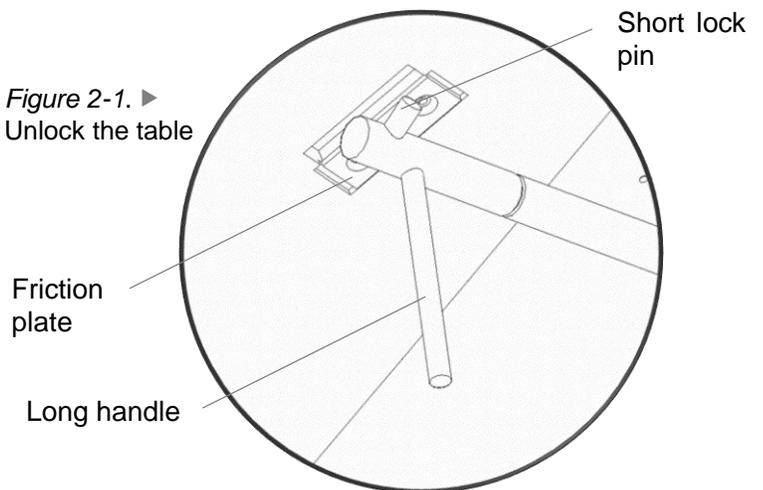
To lock the table, rotate the long handle on the lock mechanism till the short lock pin engages with the friction plate (*Figure 2-2*).
