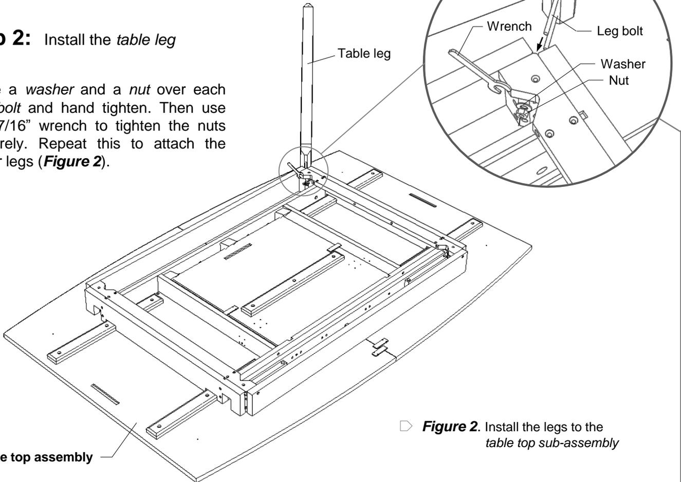
▷ **Figure 2.** Install the legs to the table top sub-assembly
