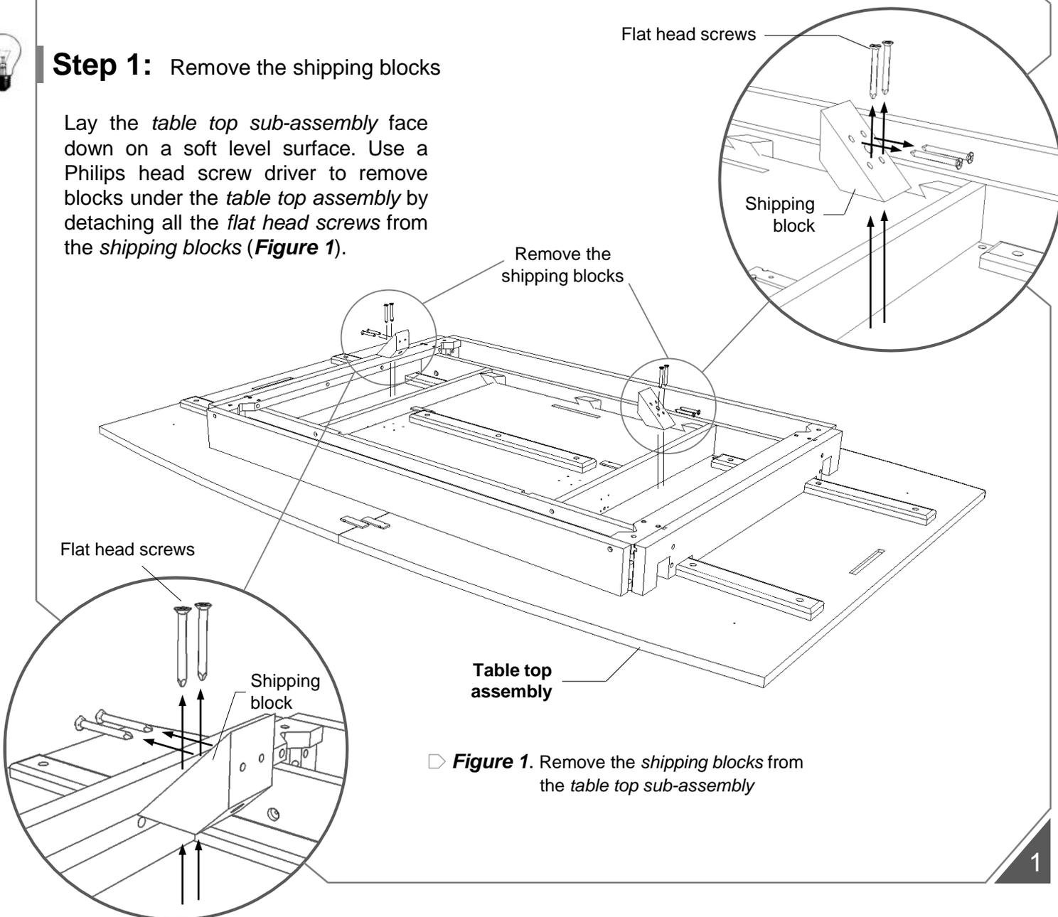
**Figure 1.** Remove the *shipping blocks* from the *table top sub-assembly*
