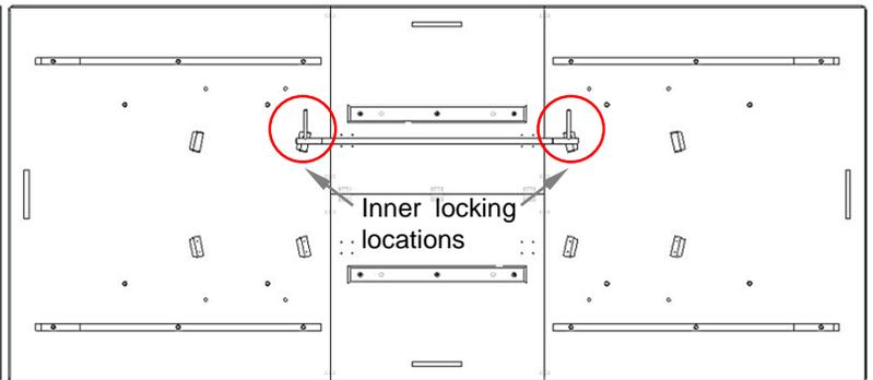
Figure 1-2. Inner locking position when leaf unfolded
