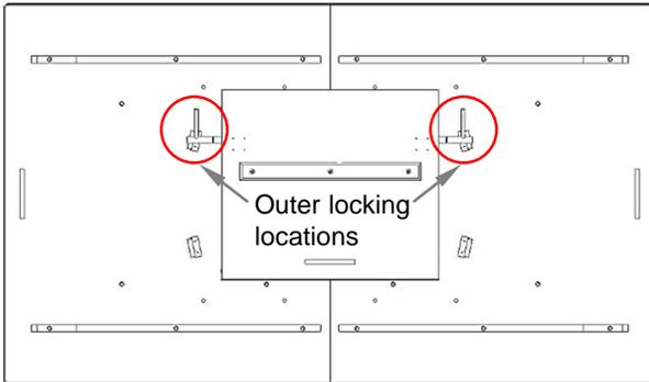
Figure 1-1. Outer locking position when leaf folded
