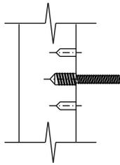
Screw the threaded stud into the insert in the *headboard leg* until it stops.
