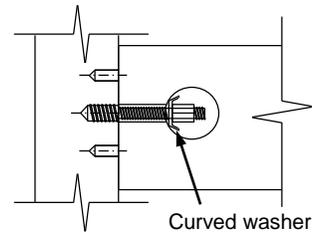
Slide the curved washer and the nut in place as shown, and tighten the nut with the wrench provided in the *side rail hardware kit*.
