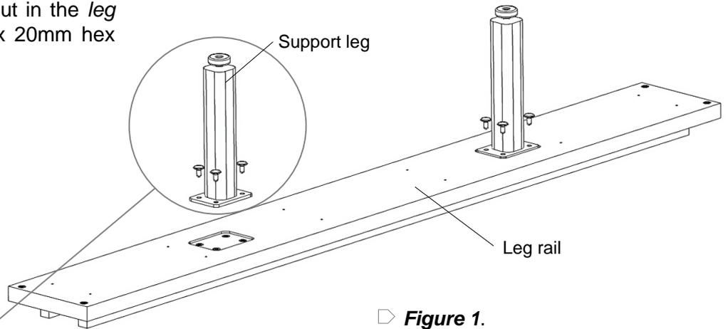
**Figure 1.** Install the *support leg* on leg rail
