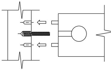
Slide the rail into mating holes for dowels on the *headboard leg*.
